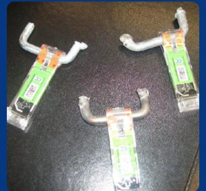
The tags are so strong that if pulled it is the metal fixing on the trolley that will often break off before the tag breaks (the average tensile strength of the tags is 120kg+).
