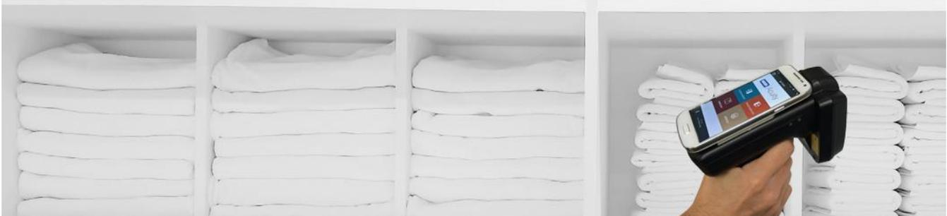
Hand-held RFID scanners can count hundreds of tags in real-time using Wi-Fi connectivity.
